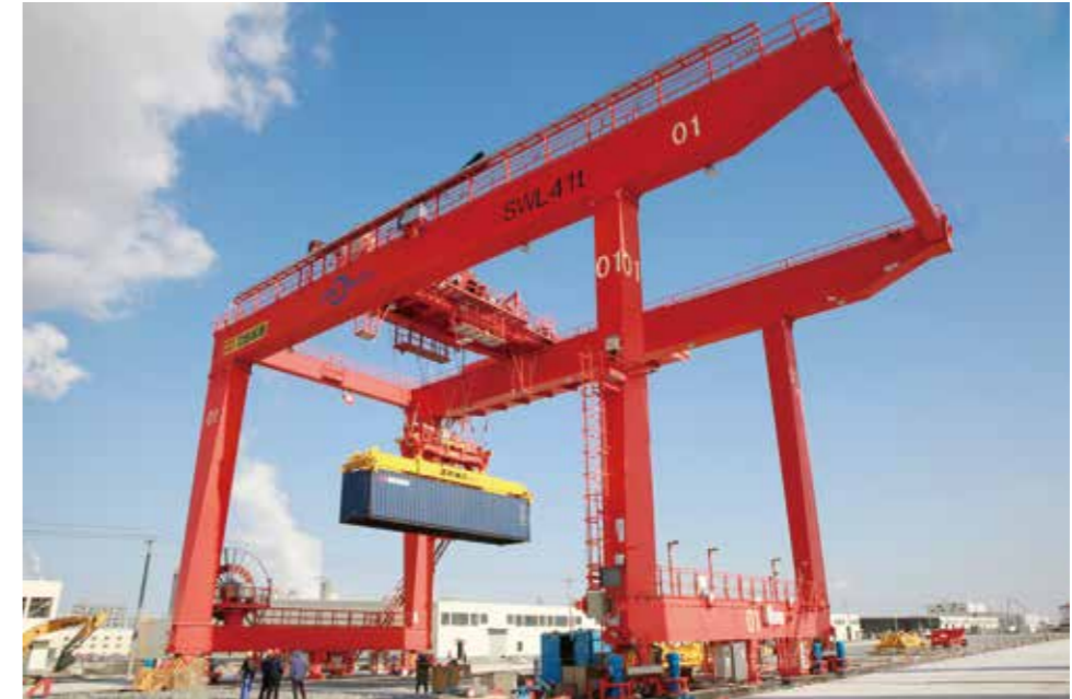
浙江石化自动化轨道式集装箱门式起重机 Automatic Rail Mounted Container Gantry Crane for Zhejiang Petrochemical Industry
