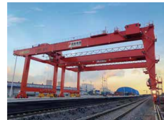
象屿集团轨道式集装箱门式起重机 Rail Mounted Container Gantry Crane for Xiangyu Group
