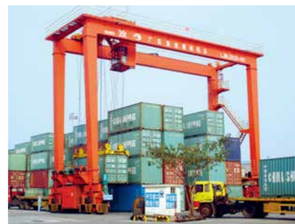
广东鱼珠穗林码头轮胎式集装箱门式起重机 Rubber Tire Container Gantry Crane Exported for Guangzhou Yuzhusuilin Wharf
